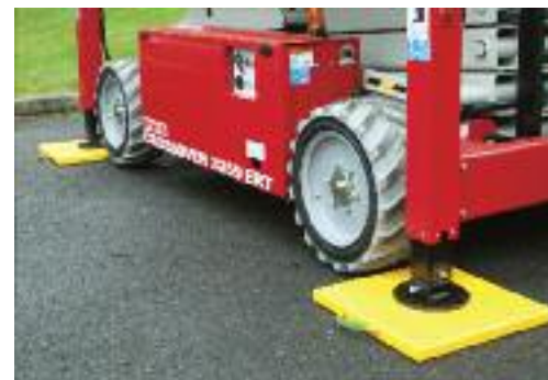
Hi-Viz outrigger pads in use on a rough terrain scissor lift.
