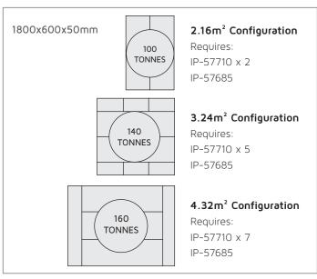
Please note: Capacity based on complete Multi Mat system. These configurations are calculated for the max ground pressure of 5kgs/cm², for normal operational conditions.
