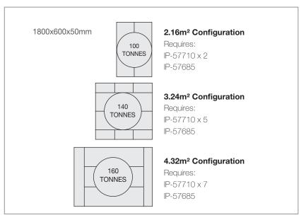
**Please note:** Capacity based on complete Multi Mat system. These configurations are calculated for the max ground pressure of 5kgs/cm<sup>2</sup>, for normal operational conditions.
